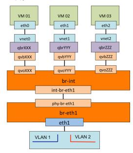
Fig. 1: OpenStack network architecture [3] on a physical host.
